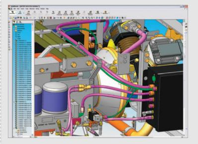
Automated documentation – Automatically create engineering drawings and bills of materials with complete information, including cut lengths for pipe and tube routes.
